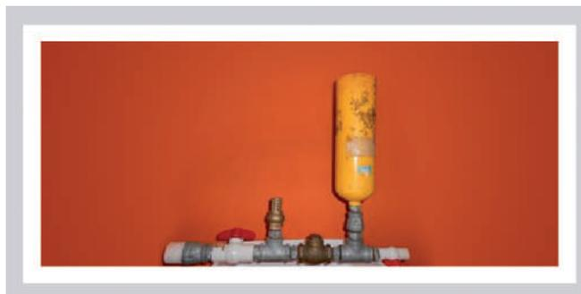
**The bike-pump (BP).** The BP operates with the simple pedaling of a stationary bike that converts mechanical energy into hydraulic energy. The operating range of the BP (Figure 6) is up to a 8m depth in the suction and up to 20m high in the discharge. The pumping rate can be from 0.8 l/s for 1m of elevation with a 1 inch hose, up to 0.2 l/s to 20m in height.
