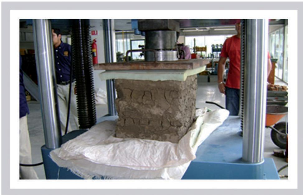
**Figure 5.** Compression test of adobe stacks
