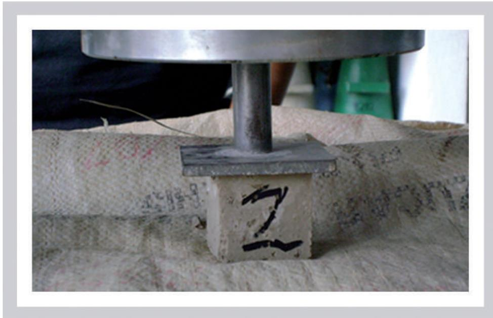
**Figure 6.** Compression test on clay mortar specimens
