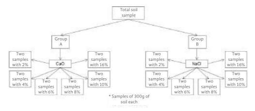
Image 2. Samples with different CaO and NaCl proportions
