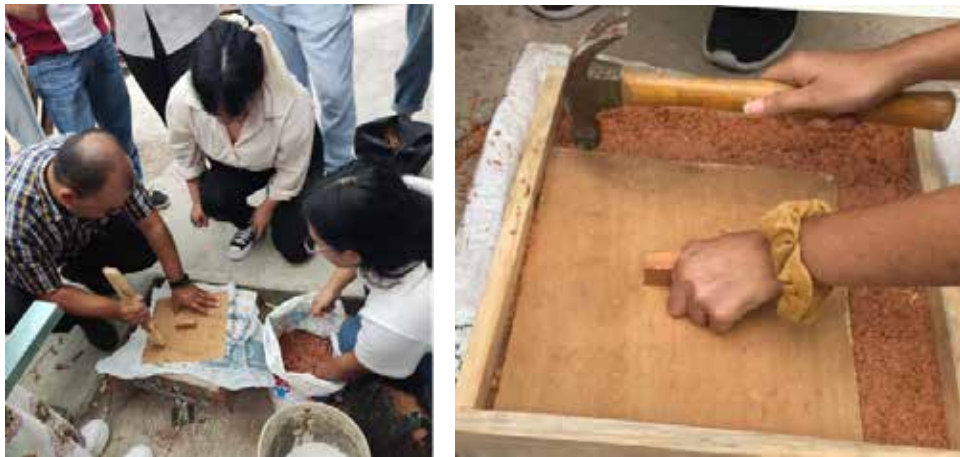
Figure 13. Preparation of sawdust panel, a product of Mount Sinai sawmill
